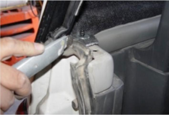
13. Cut the rear door seal flush with the hardtop. Check the tail gate for clearance in both corners, by slowly closing the gate, to ensure that nothing is touching.
