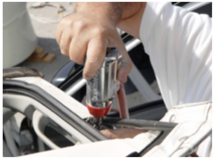
2. Remove the front soft top. Disengage the two black front clips above the windshield. Fold the soft top back and remove the screws holding the swing arm. Then disengage the rear of the soft top and remove.
