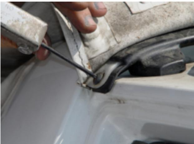
5. Using an Allen wrench, remove the two outside screws on the front section hold-down bracket. Then remove the remaining Phillips screws in the bracket and remove the bracket.
