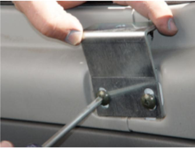
7. Install the hold down bracket. It has slotted screw holes. Loosely tighten the screws with the bracket at the upper end of it's travel, using the screws that you removed.
