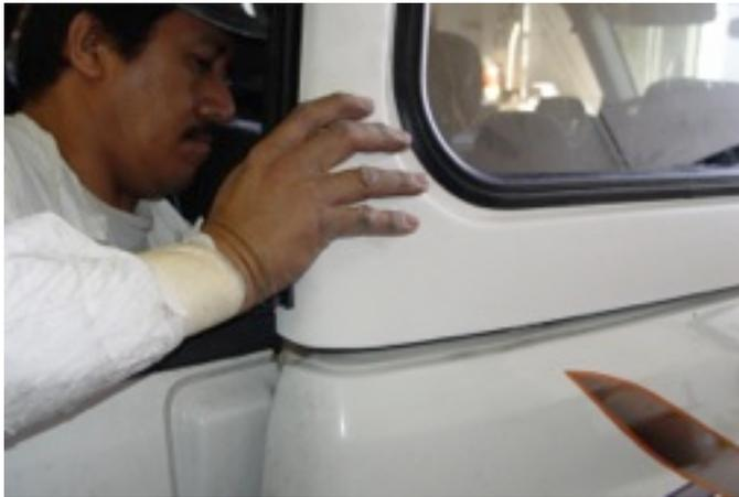
9. Remove the seal seen in #11 from under the top. Push at the rear of the top forward and down to set the top in place. Do one side at a time.
