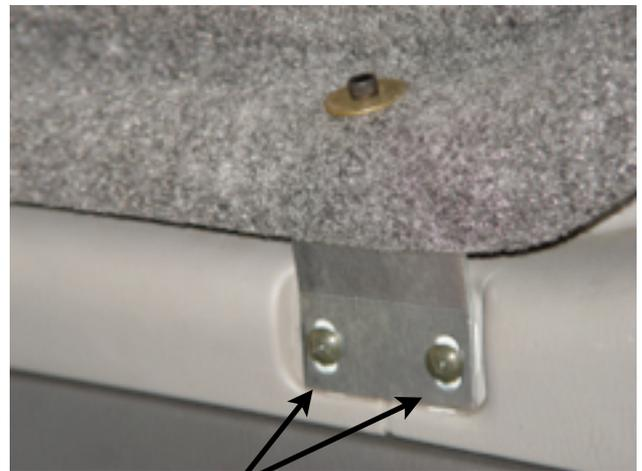
12. Now tighten the two phillips head screws on both sides,
