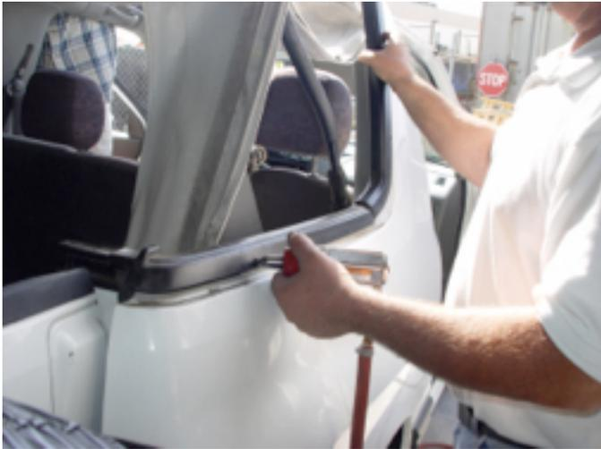
3. Remove all of the perimeter plastic hardware, with a screw driver.
