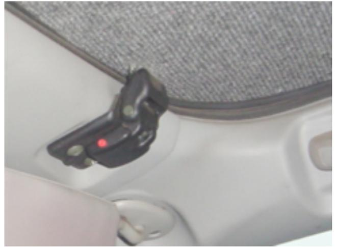
14. Using two people install the front section. Make sure the top is placed evenly on the sides. Engage the front camlock, using moderate pressure. If they are too tight follow the step 16.
