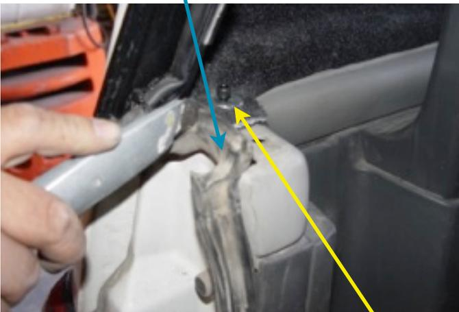
11. Install the rear socket cap screws on each side, using the 1.0" flat washers. Now tighten them and the two front socket head bolts from step 10.
