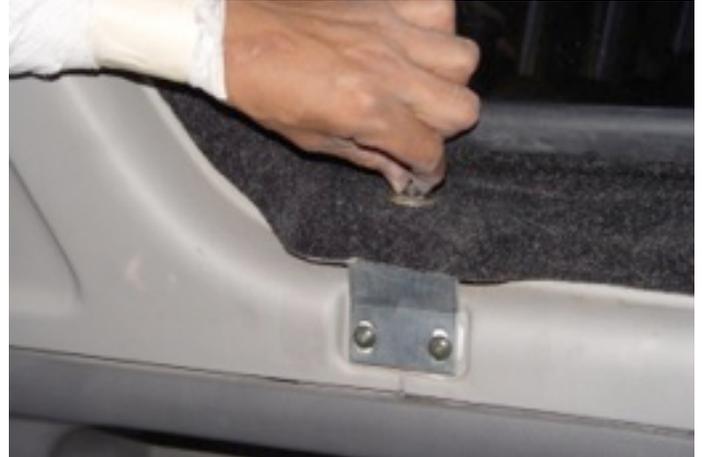
10. Install the front socket cap screw using two 1.2" flat washers on each bolt. Do both sides, but don't tighten.
