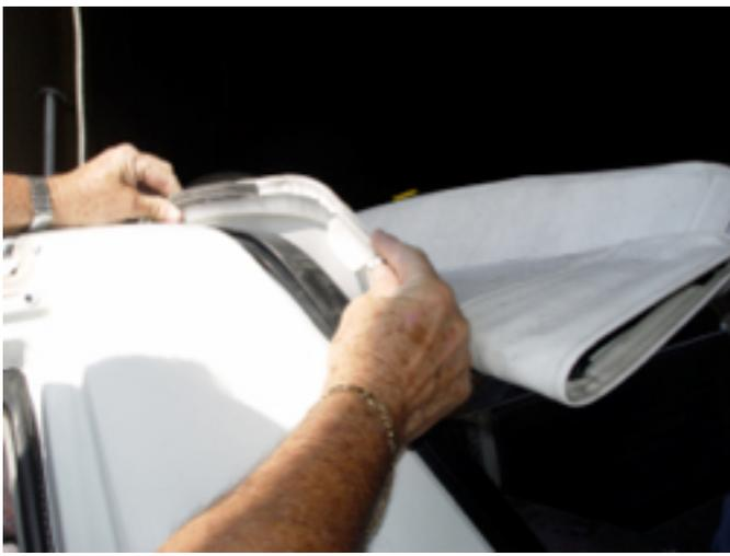
1. Remove the rear soft top. First unzip the side windows. Then pull down on the rear corners to disengage the soft top. Then disengage the front of the soft top and remove.
