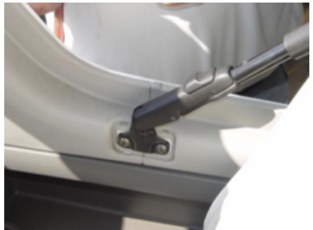
6. Remove the plastic covers from the rear bow assembly. Now remove the screws holding the bow assembly and then remove the bow assembly. Save the screws.
