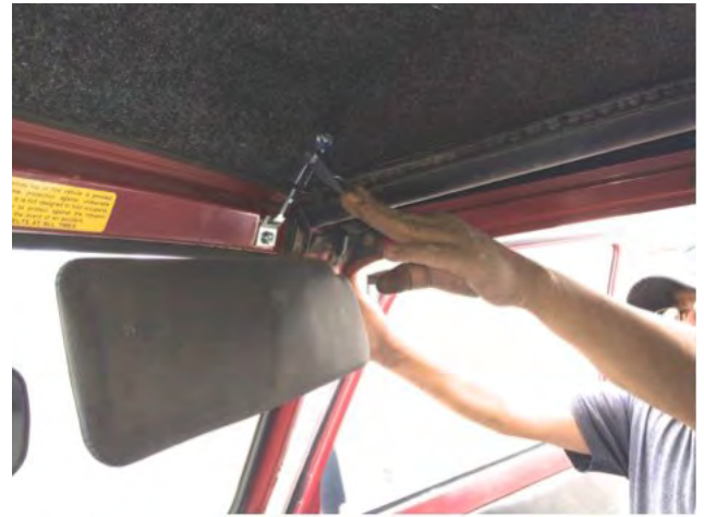
8. Engage the cam locks to medium tension.
