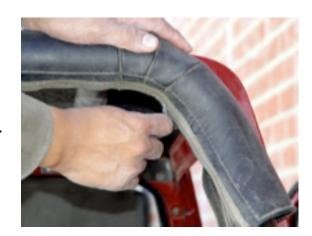
21. Install foam tape to corners. Then cut 2" of the channel, off one end of the long seal. Leaving 2" of bubble.
