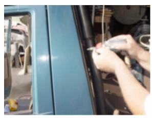
3. Install catch in factory holes in windshield frame.
