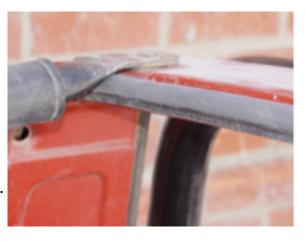
10. Remove the screw holding the roll bar support & move it to the side about 3".
