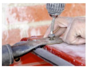
11. Apply sealant under where the roll bar normally sits.
