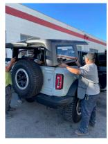
11. Using at least 2 people install the rear section on the vehicle. Push it forward and install the flange bolts. Run the bolts in, but not tight.
