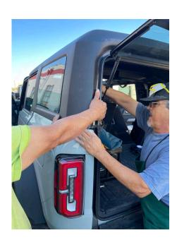
18. Now start with the rear flange bolts. Pull the top out and match the outside body line. Then tighten the rear bolt.
