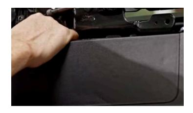
6. Remove the access panel above the rear wheel wells in the cargo area.
