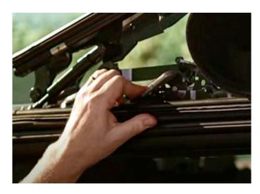
4. Above the drivers window. Press down on the latch to release the soft top.
