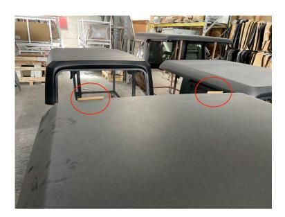
15. Install the spacers between the front and rear sections. This will keep the proper alignment between the tops.
