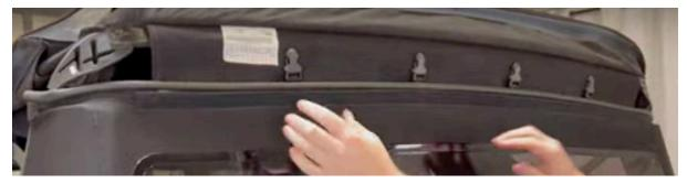
3. Remove the back window. Release the velcro along the top of the window and flip it up. Fold the bottom corners back to disengage the clips. Now remove the top corners from the slot. Unbuckle the 4 clips at the top and slide the bottom of the window out to the left of right.
