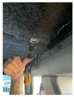
16. Engage the rear side clamp to medium tension. To adjust the tension. Open the clamp and turn the hook in or out.
