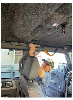
17. Now do the same with the center clamp. Engage the center clamp to medium tension. To adjust the tension. Open the clamp and turn the hook in or out.
