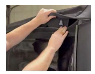
Remove the side windows. Release the velcro at the top of the window. Pull the top rear out of the slot. Unbuckle the three clips at the top and slide the window out towards the front.
