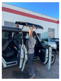
20. Undo the front section clamps front and rear. Then lift the front section off. Collect the spacers. Then tighten the mid body bolts. Then reinstall the front section and secure the clamps front and rear.
