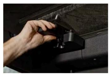
1. Release the 2 front clips. Push the soft top up and over towards the rear of the vehicle.
