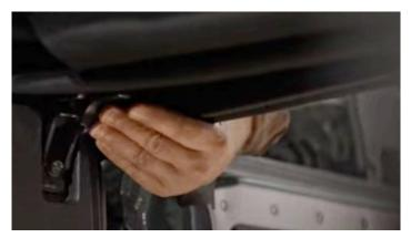
8. Push up on the latches on each side of the rear corners the soft top. This will release the soft top for removal.
