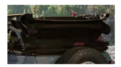
5. Lift the soft top up and to the rear of the vehicle. Press down on the soft top on both sides to latch it.
