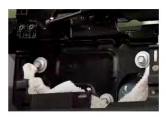
7. Place a rag in between to catch the bolts if you drop them. Using a13mm socket wrench remove the three bolts from both sides.
