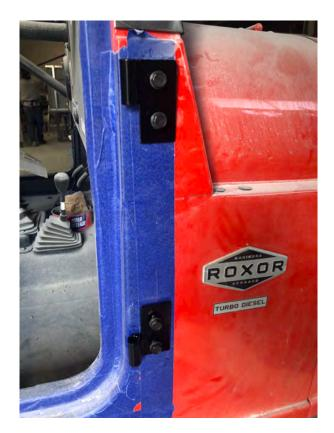
5. Install the hinges using the supplied bolts and tighten.
