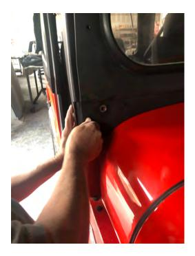
14. Reinstall the lower windshield bolts. The 3 top bolt holes will have to be drilled through the hardtop. Drill the holes and reinstall the bolts.
