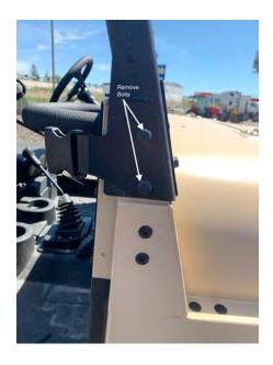
1. On the roll bar corner bracket. Remove both bolts and save them. Do both sides for all left and right instructions.
