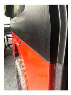
9. Go to the inside of the top and mark the 2 holes on each side for the flange bolts.
