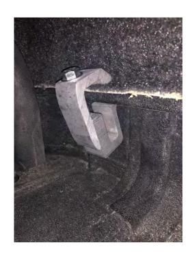
19. Install the clamp on the rear flange. Get is almost tight and then pull the rear of the hardtop out until it is flush. Then tighten all the way. See adjacent picture.
