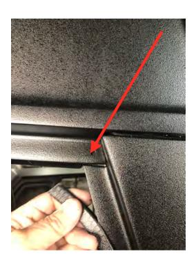
15. Locate the mark where the A pillar and hardtop meet.
