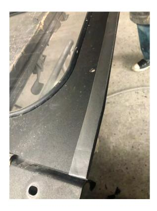
12. Now lets go to the windshield and clean the perimeter of the inside edge of the windshield. Now install the new seal.
