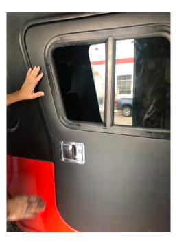
18. Adjust the door. It might be necessary to loosen the hinge bolts on the vehicle to get the door adjusted. Don't move the hinge that's on the door.
