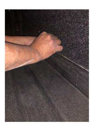
13. Install the nut plates and tighten the 4 bolts.
