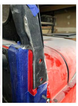
2. Using a grinder. Grind the metal end of the roll bar until it's flush with the body. See the 2 pictures on the right.
