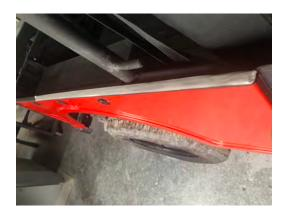
7. Lay a piece of 1" masking tape about 33" on the flange rail.
