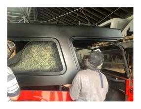
8. Install the top. Make sure the top is flush with the side of the vehicle.
