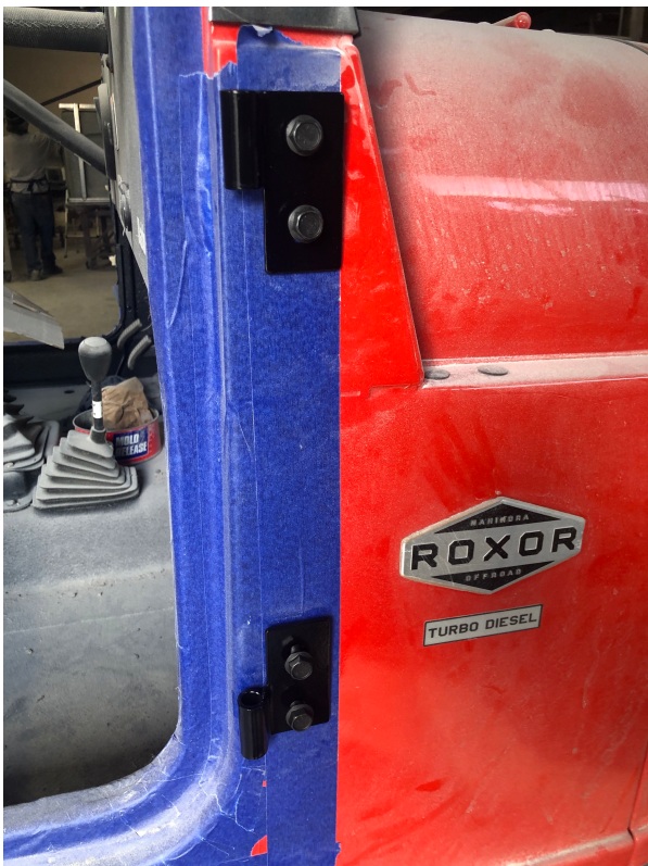
5. Install the hinges using the supplied bolts and tighten.
