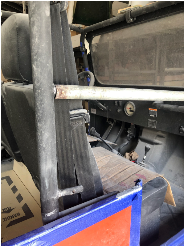
3. Using a 1" water pipe or a pipe wrench, bend the tabs on the roll bar inward.
