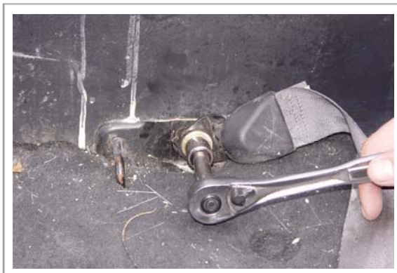
11. Remove the bolt holding the seat belt anchor and remove the seat belt mechanism totally.
