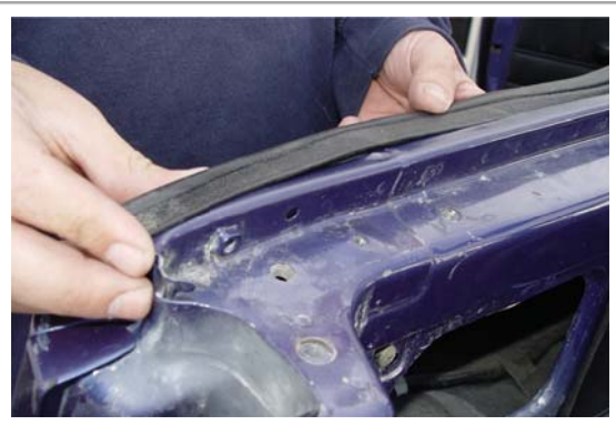
17. On 95-98 models install the supplied perimeter gasket. 89-94 models should already have a factory gasket.
