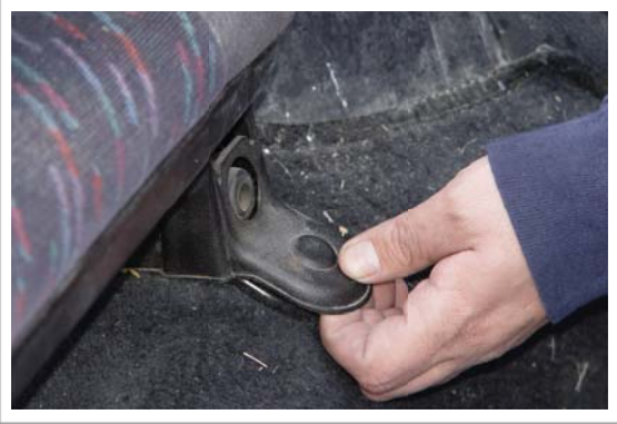
13. At the front of the rear seat, lift off cover to expose the mounting bolt.
