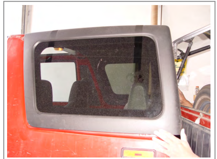
12. Now lower the back into place. Ensure the tower cover is on top of the hardtop flange. See step 14.
