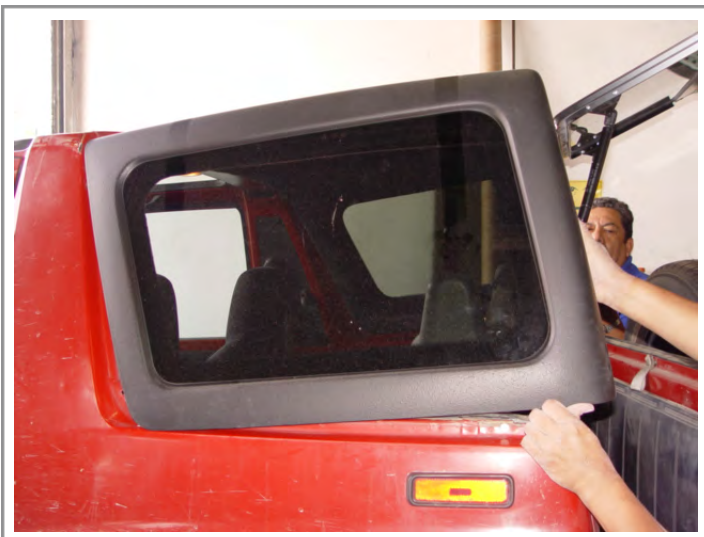
11. Using 2 people, open the rear hatch, place the top on the vehicle, as shown. This engages the front flange.
