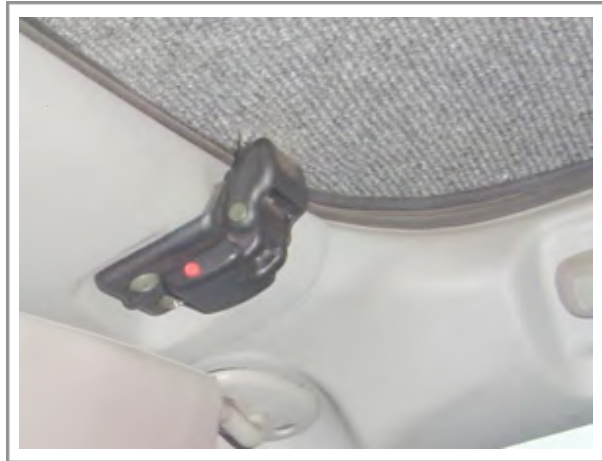
3. Insure that the factory clamps are in good condition. Install front section, so that the front factory clamps are centered in the front section's catches. Push down on the front section and engage the clamps into the catches. Only use medium pressure. If needed adjust the hardtop catches by clamping them with a vise grips and gently pulling down on them to open them up a little.
