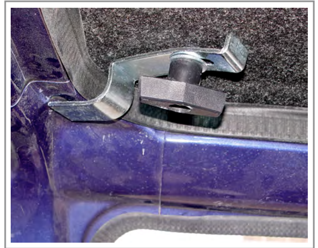
4. Attach the rear clamp using the 5/8" washer and wing nut provided. Tighten both sides.
