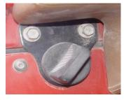
4. CJ5 Loosen the bolts and wing nut. Adjust windshield and tighten.
