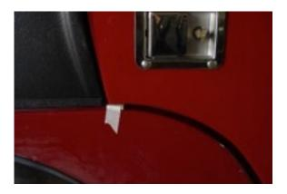
7. Using 2 people, mount the door in the opening. Make sure you have an even space around the door. Use the spacers as a guide. Now slide the lower hinge onto the door, one at a time and mark the center of the 2 holes. Remove the door and drill the four 7/16" holes in the body. Remove the masking tape from around the holes and install the hinges using the bolts from the package and the weld nuts. Now install the doors.
