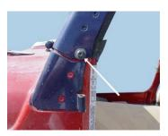
4. TJ & Unlimited-Using a T40 Torx wrench, loosen the bolt above the doors hinge. Go to step 5.
