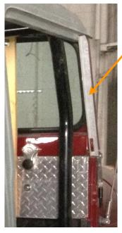
4. Install new door end plates on the side on the windshield. Using the double sided tape and the existing screws.
