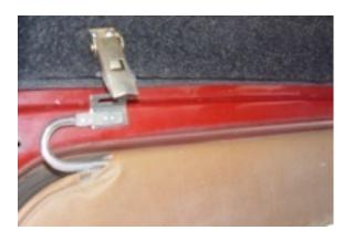
3. With the top in the proper position, drill a small pilot hole directly below the front camlok. Install catch using supplied screw.
