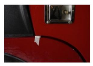
4. Tape spacer to the rear of the door opening.
