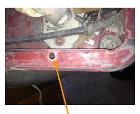
2. Install the top on vehicle. Use the large bolts in the front holes. Try and use the large bolts in the rear holes. If they don't work use the small bolts. Do not tighten bolts all the way.
