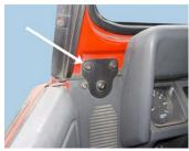
4. CJ7 - CJ 8 - YJ Loosen bolts using a T40 torx wrench.
