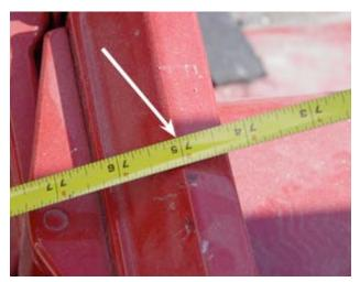
3. Where the tape hits the body, it should read the value in the chart below. Measure both sides. If it does, put the top on. If not, go to step 4.
