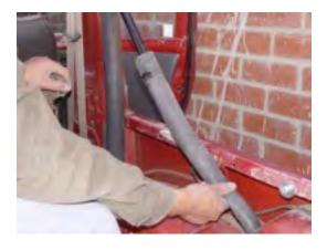
17. Remove the roll bar side support bolts then remove the padding and reinstall the bolts.
