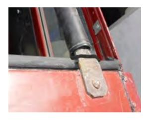
13B. Lay a bead of silicon across the bar and extend it about 2" past the bar on both sides.
