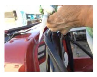
13. Seal all the holes in the front flange valley, so that any trapped water will exit outside of the cab area.
