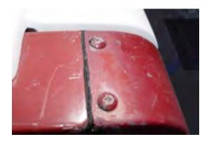
13A. Totally seal this crack starting from the bottom of the flange all the to other end.
