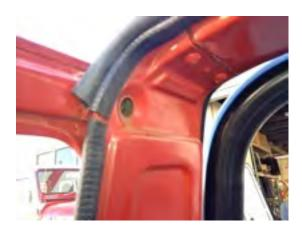
Starting at the cut end of the vertical trim. Install the new 46" front body trim piece, all the way to the other side. Cut at the other end so that it meets up with the other vertical end.
