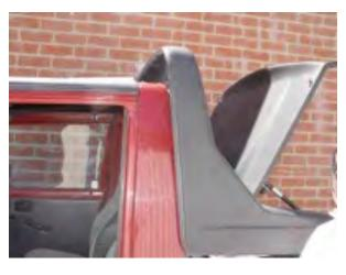
22. Using two people, place the rear section on the Samurai. It must be in the position shown and then lowered into place.
