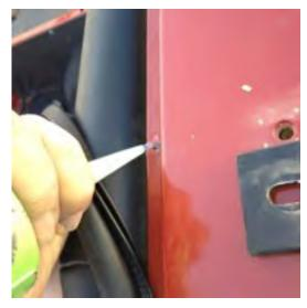
13D. Seal all screw holes and any other cracks along the sides and top.
