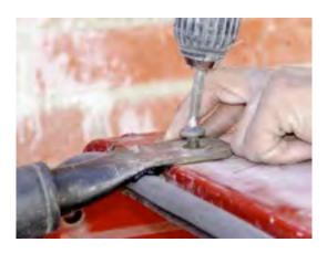
10. Remove the rear screws holding the roll bar supports and move the roll bar to the side about 3 inches.
