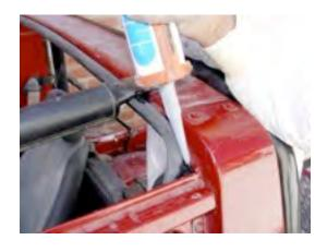
13E. Seal all the holes in the front flange valley, so that any trapped water will exit outside of the cab area.
