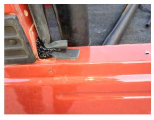
20. Now put a piece of foam in the corner and silicone the corner as shown.
