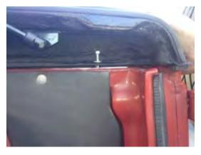
24. Install the 5/16" button head bolt and 3/8" silver washers in rear hole. Do not tighten the bolt all the way down.
