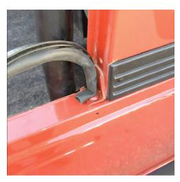
19. Start the rear seal on the flange so the bubble extends horizontal about 1.5". Then continue installing the seal on the flange. At the other, cut the seal 1.5" past the end. Then cut 1.5" off the u shape and lay the bubble flat so it looks like the other side.
