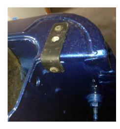
21. Install the bracket in the rear mounting hole. Then secure using the 2 supplied screws.
