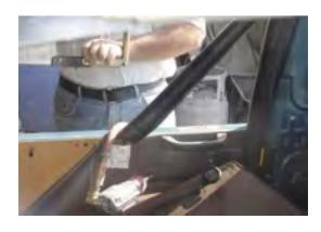
2. Remove rear bow screws & remove bow assembly.
