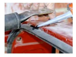
11. Using the supplied sealant, apply sealant under where the roll bar sits when it is screwed in.
