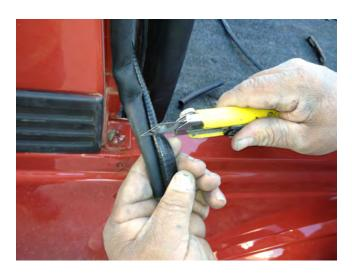
18. Cut the u shaped channel off the end of the seal about 1.5" from the end.
