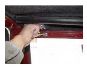
Install flat latch hook (notch facing down) on door jam rear factory hole, using M6 x 20 screws.
