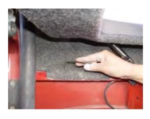
23. Install the forward M6 x 30 button head cap screw and 1.25" cut washer.
