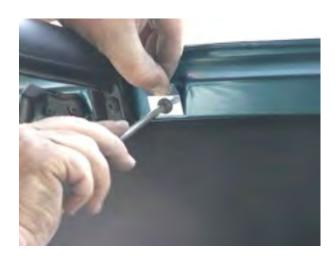
4. Install angled latch hooks in factory holes in the windshield frame using M6 x 20 screws.
