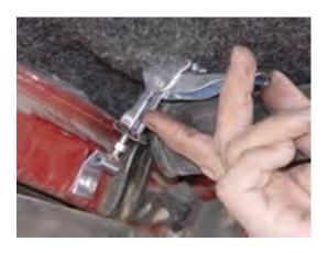
26. Install the front section and secure the cam-locks. Latch the side cam-locks first and then the front ones. Cam-locks should be adjusted for medium tension.
