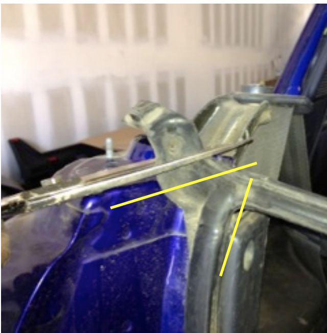
10. Cut back door seal on the yellow line. Both sides.
